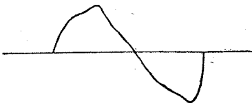
Fig. 9. Observed output waveform for a DC input of 100mV.
